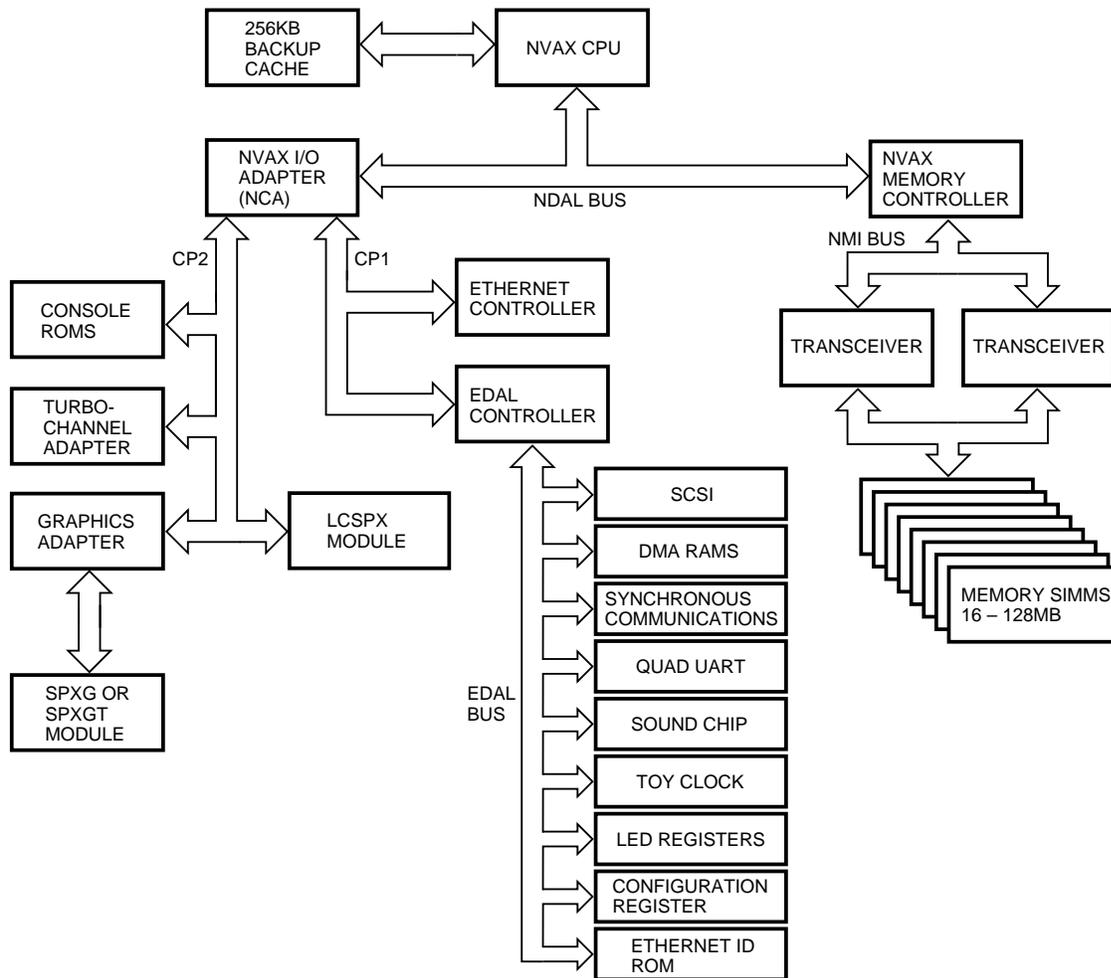
Figure 1 Block Diagram of the VAXstation 4000 Model 90
